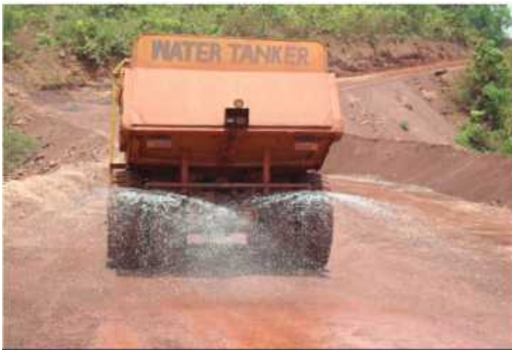
PHOTO # 1 SHOWING THE WATER TANKER ON HAULAGE ROAD FOR DUST SUPPRESSION
